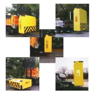
U-MAD Truck Mounted Attenuators (TMAs) offer outstanding perfomance to supply protection for workers, motorists and equipment. The U-MAD is available in two styles, TL-2 or TL-3, depending on workzone speeds. The TMAs are designed to absorb collision energy during rear-end impacts, prevent impacting vehicles from underriding the truck and reducing expensive damage to equipment.
